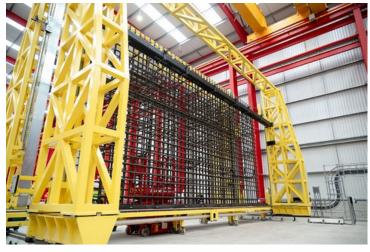
A new factory in Avonmouth near Bristol is helping to extend the use of "Modularisation", a construction method whereby large items such as tanks, pools and sections of steel reinforcement are built as complete structures in 'satellite' factories close to the Hinkley Point C construction site.
